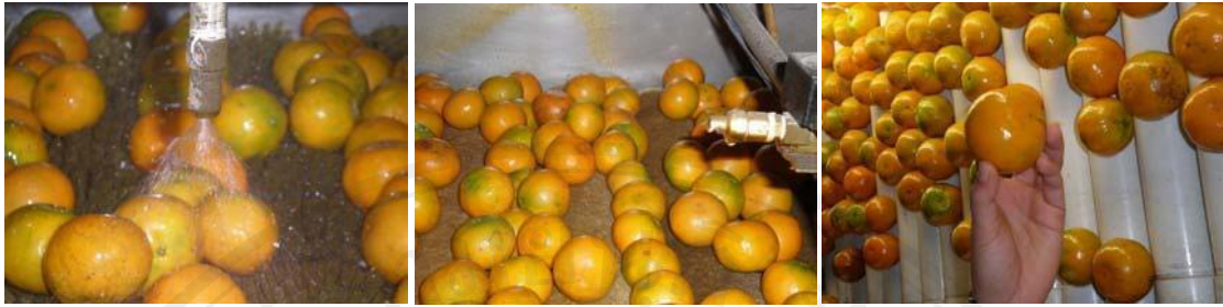
Figure 3.9 Cleaning and coating application by commercial method
