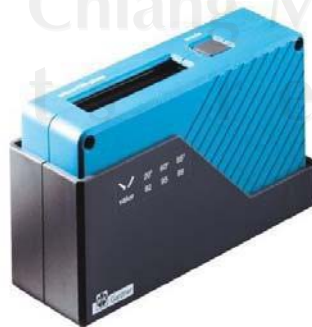
Figure 3.10 Micro-TRI-gloss reflectance meter (BYK Gardner Inc., MD, USA)
