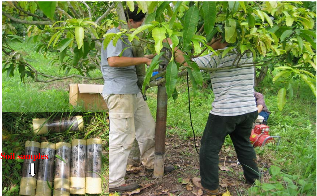
Figure 9.4 The soil samples in B plot are collected by cylindrical-drilling machine.
