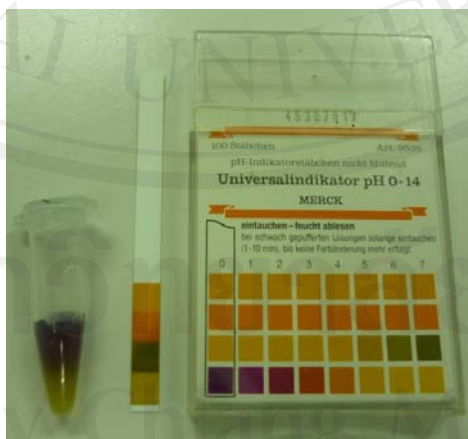
Figure A.8 Test pH with positive control (low concentration) by pH paper
