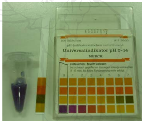
Figure A.7 Test pH with positive control (high concentration) by pH paper
