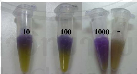
Figure A.5 10, 100 and 1000 \mu\text{g}/\text{kg} antibiotics and negative control of normal test kits
