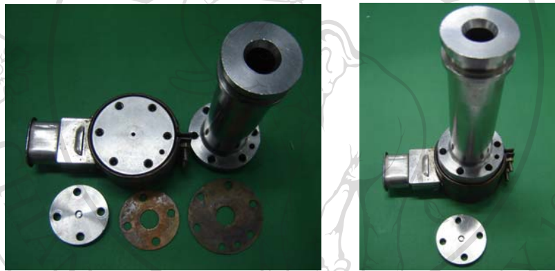
Figure 2.19 The various accessories used in the fabrication of small tubes by melt extrusion.
