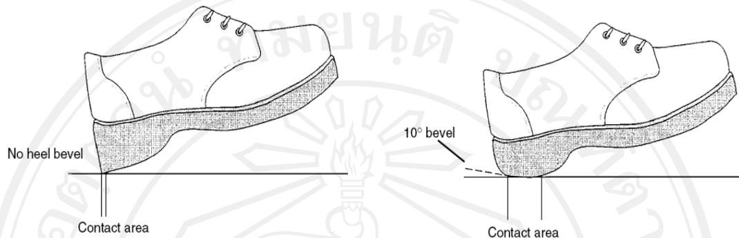
Figure 4 Bevelled heel shoes (14)
