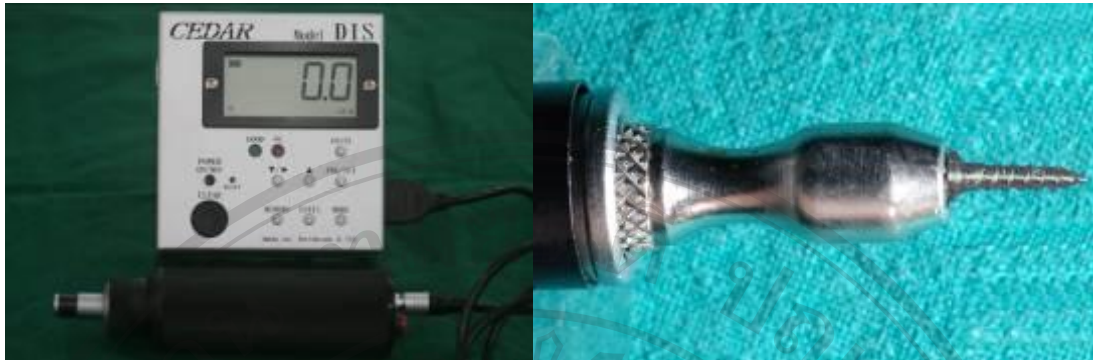
Figure 4.4 A. Imada torque wrench (DIS-RL, Imada Inc., Northbrook, USA). B. Jacobs chuck of the torque wrench for applied to the miniscrew.
