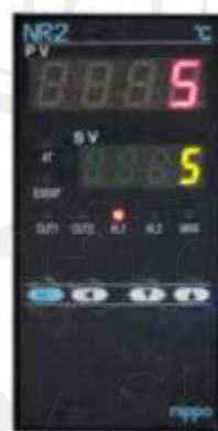
Figure 35 a. Thermocycling machine set at 2,000 cycles, b. Cold-water bath set at 5° C, and c. Hot-water bath set at 55° C.
