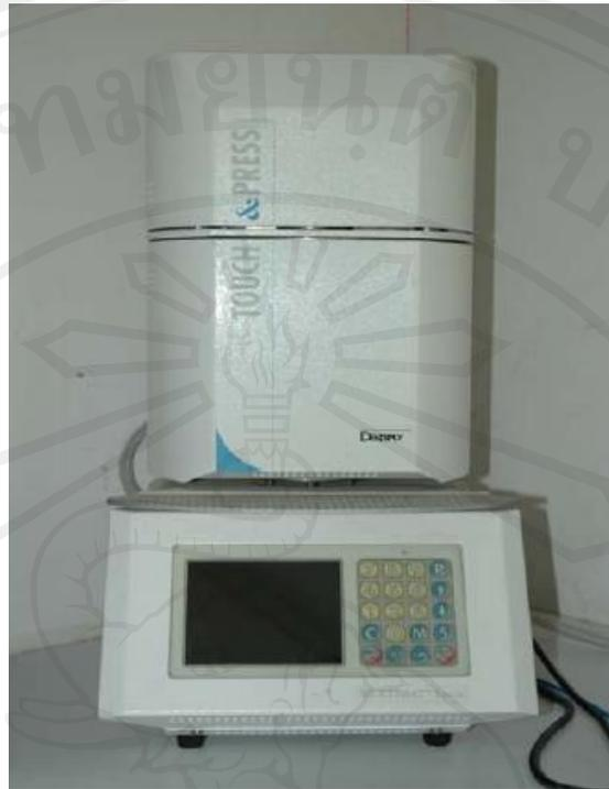
**Fig. 3.3** Vacuum furnace (for reducing sample porosity after sintering process).
