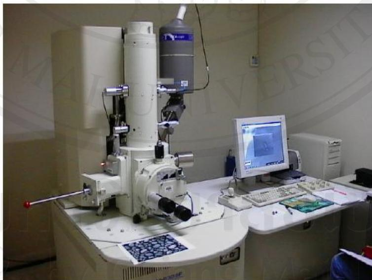
**Fig. 3.7** Scanning electron microscope, equipped with EDX analyzer.
