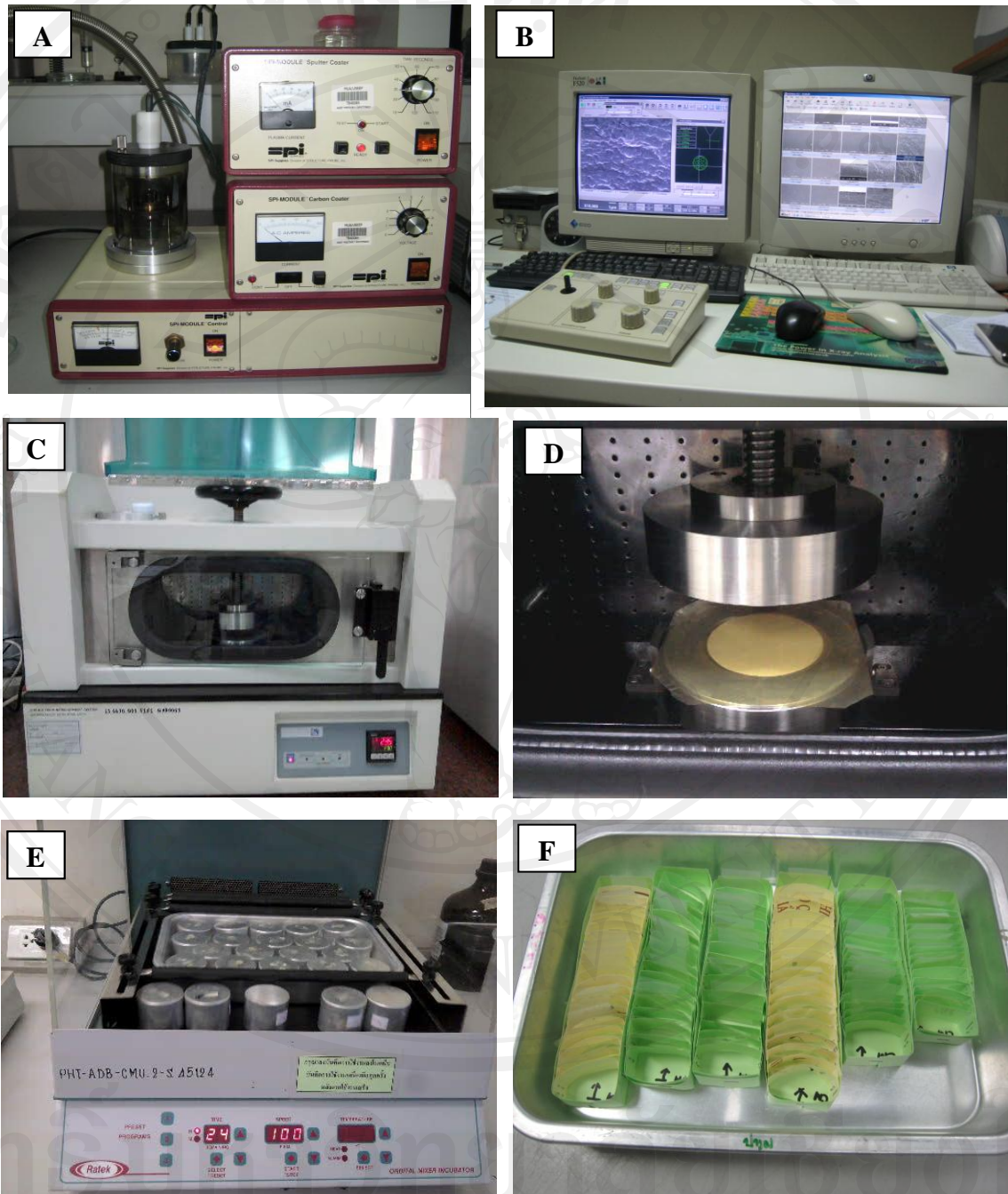
Figure 4.2 The equipments were used to determine film properties included: (A,B): scanning electron microscope system; (C,D) oxygen permeability; (E): solubility and (F) prepare film samples for sorption isotherms determination.
