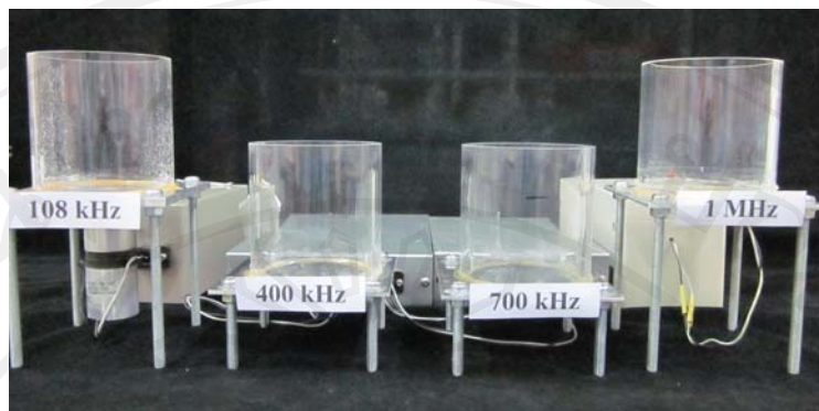
Figure 3.1 Ultrasonic devices at 108, 400, 700 kHz and 1 MHz.
