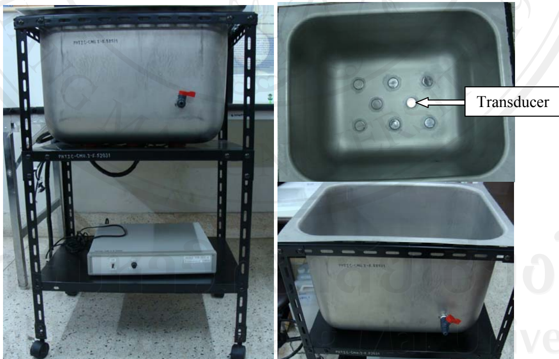
Figure 4.1 Ultrasonic device at 1 MHz for chilli washing.
