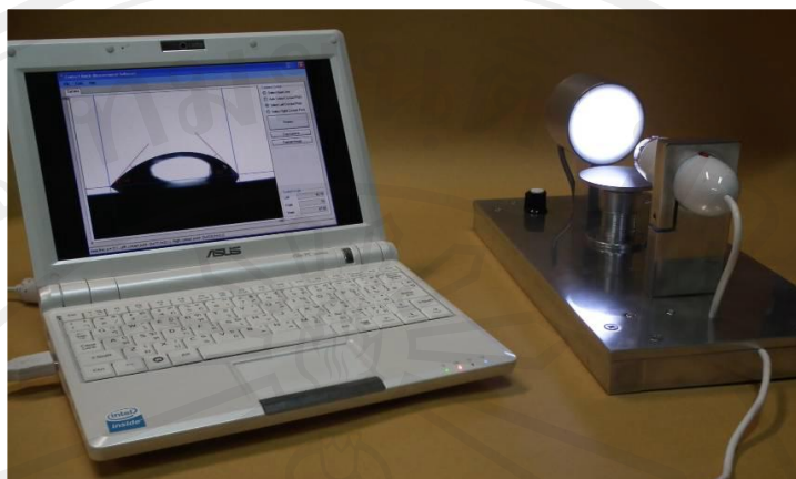
Figure 2.3 Contact angle measurement at PBP laboratory, Physics and materials science Department, CMU.
