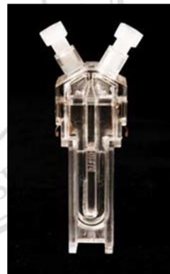
Figure 21 Equipment of Zetasizer. a) Particle size analyser Malvern (Zetasizer ZS) b) Disposable plastic micro cuvette (ZEN0040) for measuring PDI and size of nanoparticles. c) folded capillary cell (DTS1070) for measuring zeta potential of nanoparticles.
